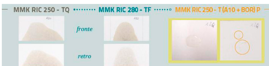
Figure 4. Comparison between the level of absorption of uncoated paperboard (sx), fluorinated paperboard (c) and natural-based coatings (dx) on recycled paperboard
