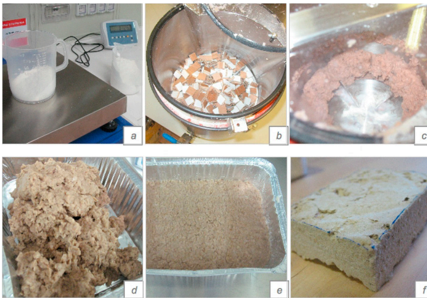
Figure 1. Productive phases: weighing the right amount of PCMs (a), waste paper (b) and water; pulping (c) and distributing (d) the water-based solution; drying the composite material (e); obtaining the solid panel (f).
