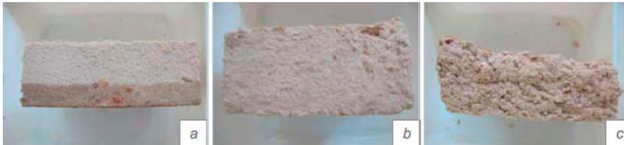
Figure 5. Partial water immersion effects on pearlite panel (a) and cellulose panel with different percentage of antihumidity additives: 15% (b) and 30% (c).
